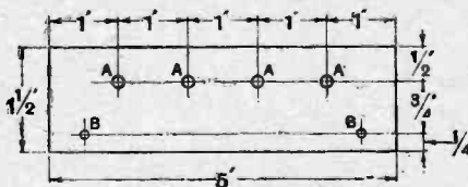
Fig. 3.—The terminal panel. A, 5/32in. dia.; B, 1/8in. dia.
