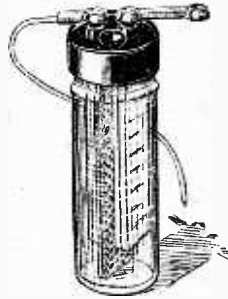
One of the cells of the Storad battery.
