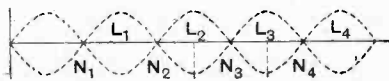
Voltage nodes N_1, N_2, \dots , and antinodes or loops L_1, L_2, \dots , of stationary electric waves on a straight wire.
